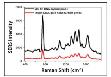
Figure 3: SERS-based detection of a segment of the HIV-1 gag-gene using popcorn-shaped gold nanoparticles conjugated with graphene oxide (black) and with the gold nanoparticle alone (red).
