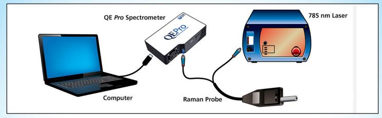
Figure 1: Modular fiber optic Raman spectroscopy system for SERS detection.
