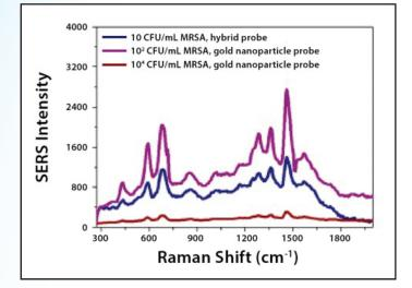
Figure 4: SERS-based detection of MRSA using popcorn-shaped gold nanoparticles conjugated with graphene oxide (purple), with the gold nanoparticle alone (blue) and with graphene oxide alone (red).
