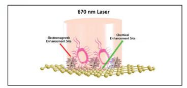
Figure 2: In a hybrid SERS probe for ultrasensitive biosensing, popcorn-shaped gold nanoparticles (spiked balls) result in electromagnetic enhancement of the SERS signal, while conjugated graphene oxide (grey mesh) provides chemical enhancement.
